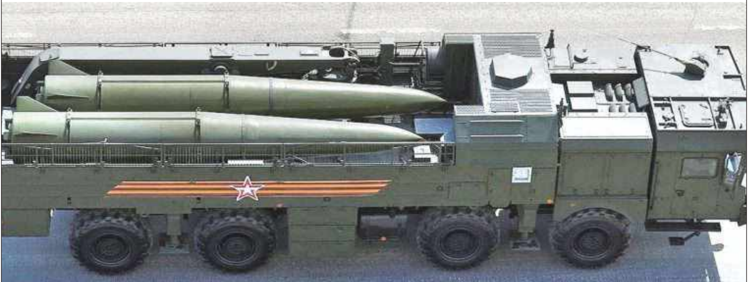
The Russian 9K720 Iskander is a mobile short-range ballistic missile system. It is replacing the OTR-21 Tochka system.
